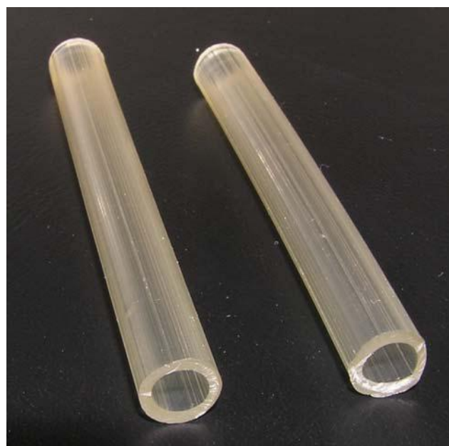
Fig. 1: Hot-melt extruded ethyl cellulose cylinders (containing 20 % dibutyl sebacate as a plasticizer)
