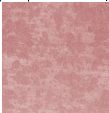
Fig. 7: Sample Immersed in 0.2% inhibitor solution
