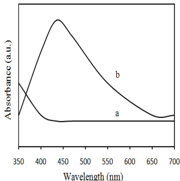
**Fig. 1: UV-Visible absorption spectra of (a). Seed extract of *Cherimoya* (b). Synthesized AgNPs**
