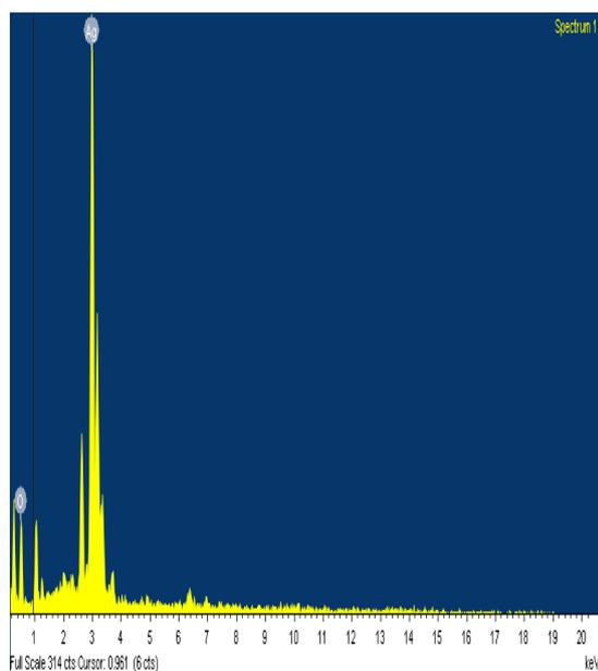
**Fig. 5: Energy dispersive X-ray spectroscopy (EDX) image of synthesized AgNPs**
