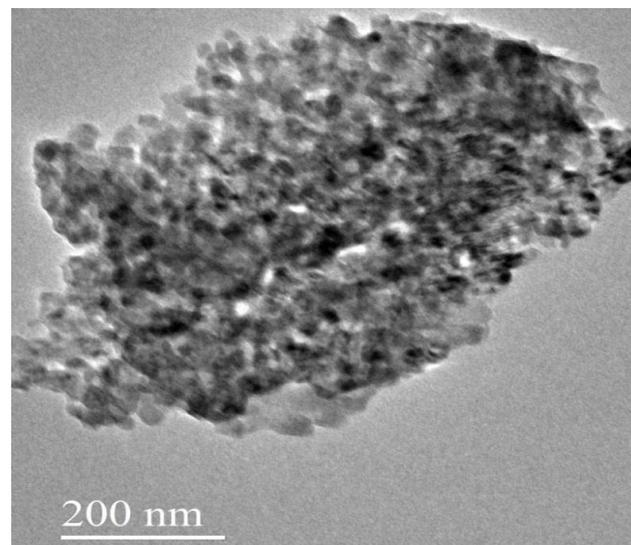
**Fig. 6: Transmission electron microscope (TEM) image of synthesized silver nanoparticles**
