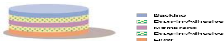
Fig.2: Multi-layer drug in adhesive
