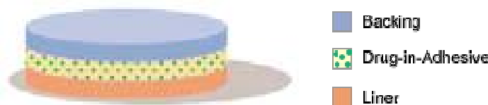
Fig. 1: Single-layer drug in-adhesive
