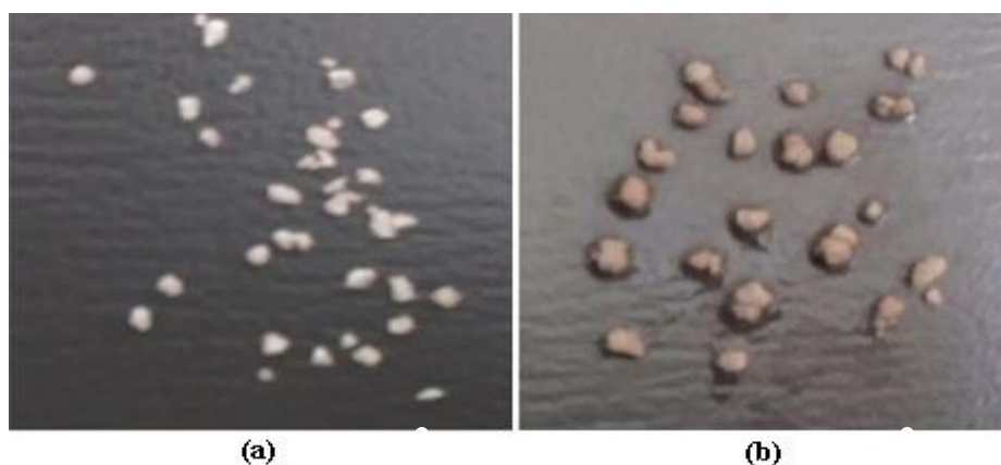
Fig. 2: Microparticles (a) Before swelling (b) After swelling
