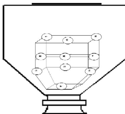
**Fig. 2: Illustrative Diagram of Conta Blender and Sampling Locations**
