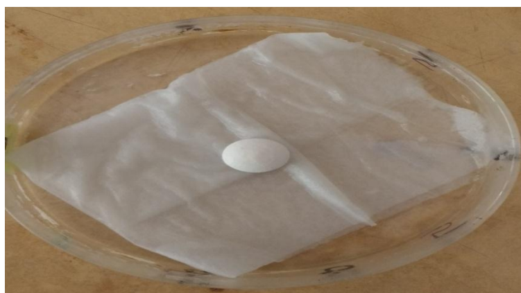
Fig. 10: Wetting time determination of Immediate release tablet
