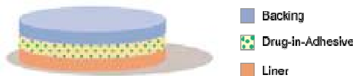
Fig. 1: Single-layer drug in-adhesive
