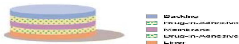
Fig.2: Multi-layer drug in adhesive
